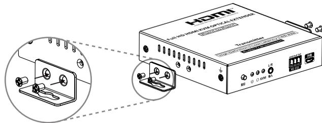
Note: Choose the wall mounting position and attach the mounting ears to the unit according to the diagram.
