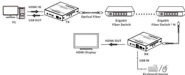
Note: It is suggested to use gigabit (1000 Mbps) switches in LAN transmission, and 100Mbps switches should not be mixed with gigabit switches when cascading.
